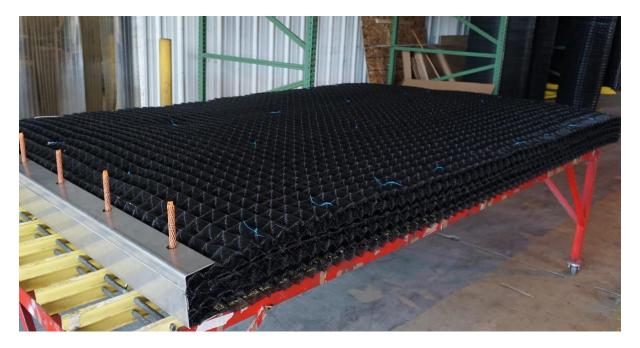
Mist eliminators or <u>demister pads</u> are used in processes or techniques wherever efficient filtration is required. In addition to filtration, they also limit product loss and prevent the equipment from getting damaged. All of this is to say that **demister pads** play an extremely crucial role in process operations.
